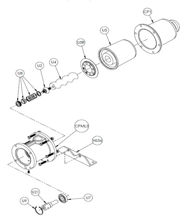
Pump bolts to any Nema Frame 56 C-Face motor with feet.
