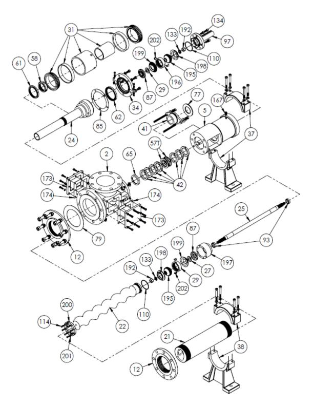
**Before starting dis-assembly**, drain lines and suction housing of as much liquid as possible. A section of the piping at the discharge side of the pump should be easily removable to facilitate the replacement of rotor, stator, or gear joint parts. The recommended "Length of Piping" is as set forth in CLEARANCE TABLE NOTE "A".
