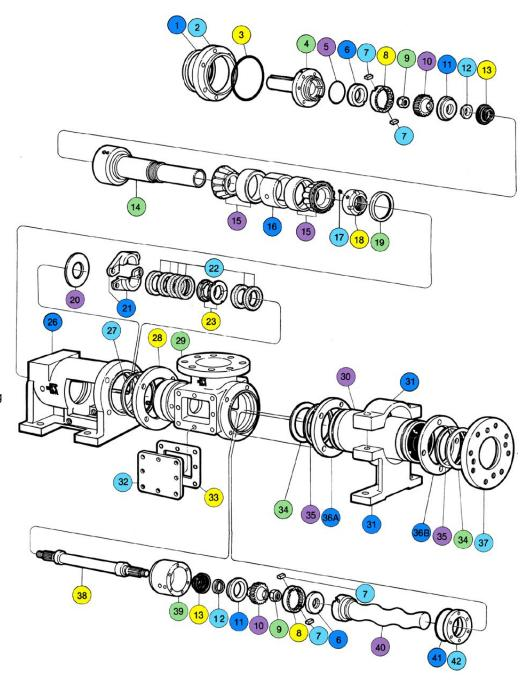
Gear Joint Kit (Includes quantiy 1 each of part (6), (8), (10), (10), and quantity of 2 of part (7).)
