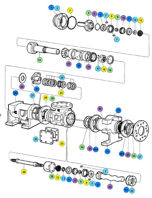
Gear Joint Kit (Includes quantiy 1 each of part 6, 8, 10, 11, 12 and quantity of 2 of part 7.)
