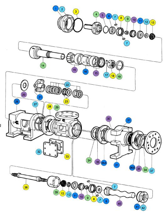
Gear Joint Kit (Includes quantiy 1 each of part 6, 8, 10, 111, 12 and quantity of 2 of part 7.)
