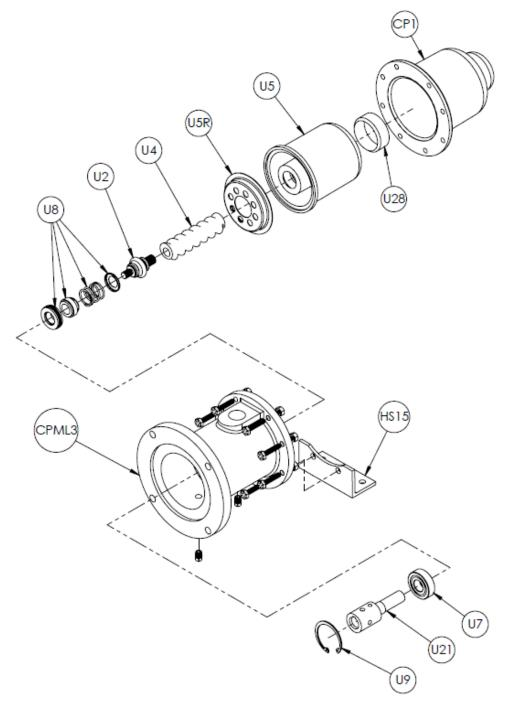
Pump bolts to any Nema Frame 56 C-Face motor with feet.
