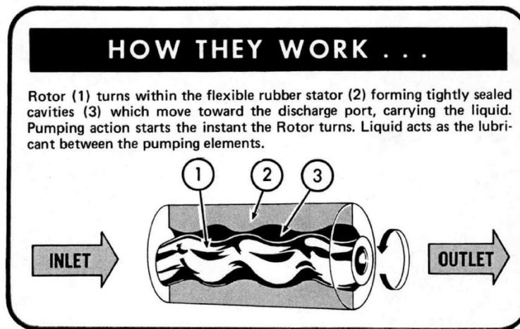
In operation our pumps are fundamentally fixed flow rate pumps and offer long life and reliable service transporting thick or lumpy fluids. However, abrasive fluids can significantly shorten the life of the stator. Also, slurries can be pumped reliably if the slurry is viscous enough to maintain a lubrication layer around the particles and protect the stator.
